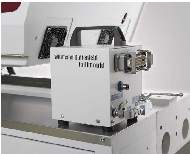
WITTMANN BATTENFELD Cellmould technology, developed to save material and reduce weight (picture: WITTMANN GROUP)
